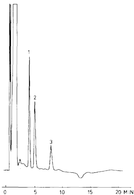
Fig. 4. Chromatogram of a plasma sample from a pig. Sampling was performed 1 h after intravenous administration of 50 mg of mebeverine hydrochloride. For chromatographic conditions, see text. (detector sensitivity: 0.02 a.u.f.s.). Peaks: 1 = mebeverine (126 ng/ml); 2 = internal standard; 3 = alcohol derivative (57 ng/ml).
